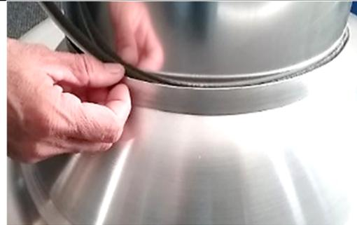
With **utility knife**, score & cut along **flashing lip** excess **tube** sticking out; edges must be flush with flashing.
