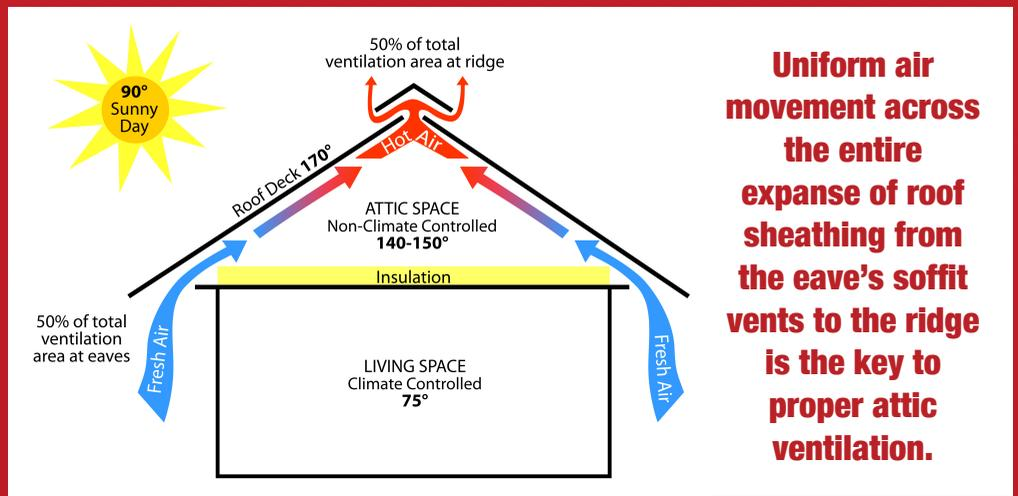
**Uniform air movement across the entire expanse of roof sheathing from the eave's soffit vents to the ridge is the key to proper attic ventilation.**
