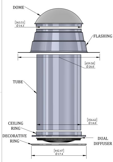
**Dome**: 100% high-impact clear acrylic, formed and sealed onto aluminum ring. Designed to protect dome edges and expel any condensation build-up during winter months. Inner prismatic dome helps catch low angle rays and scatter sunlight before entering tube.
