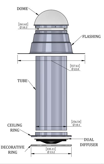
**Dome**: 100% high-impact clear acrylic, formed and sealed onto aluminum ring. Designed to protect dome edges and expel any condensation build-up during winter months. Inner prismatic dome helps catch low angle rays and scatter sunlight before entering tube.
